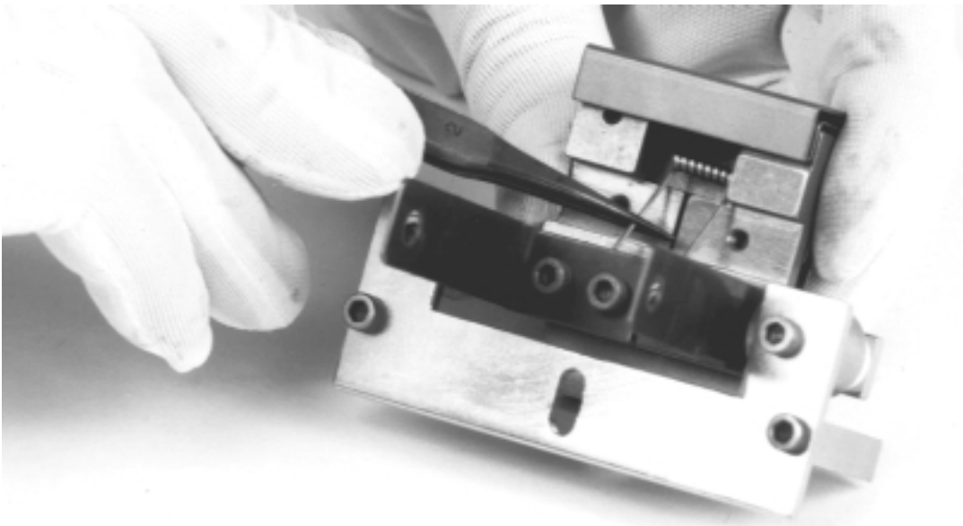
Figure 4-3. Removing the filament
