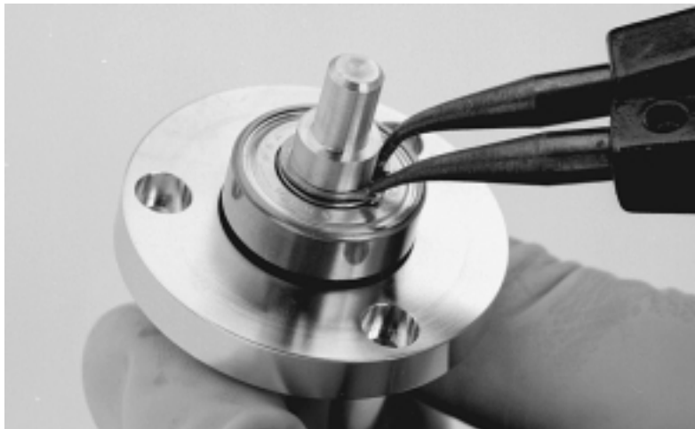
Figure 6-31. Removing the retaining ring that retains the drive shaft
