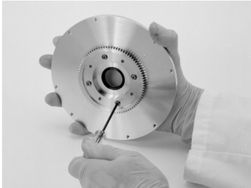
Figure 6-25. Removing the ring gear from the crucible mounting flange
