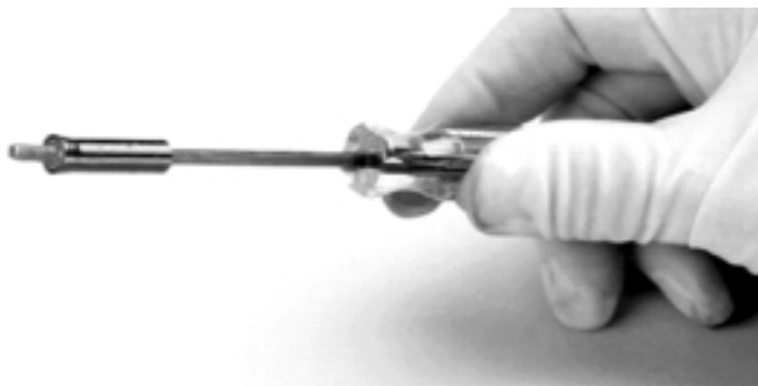
Figure 3-5. Socket-head screw correctly retained by sleeve on end of Allen driver
