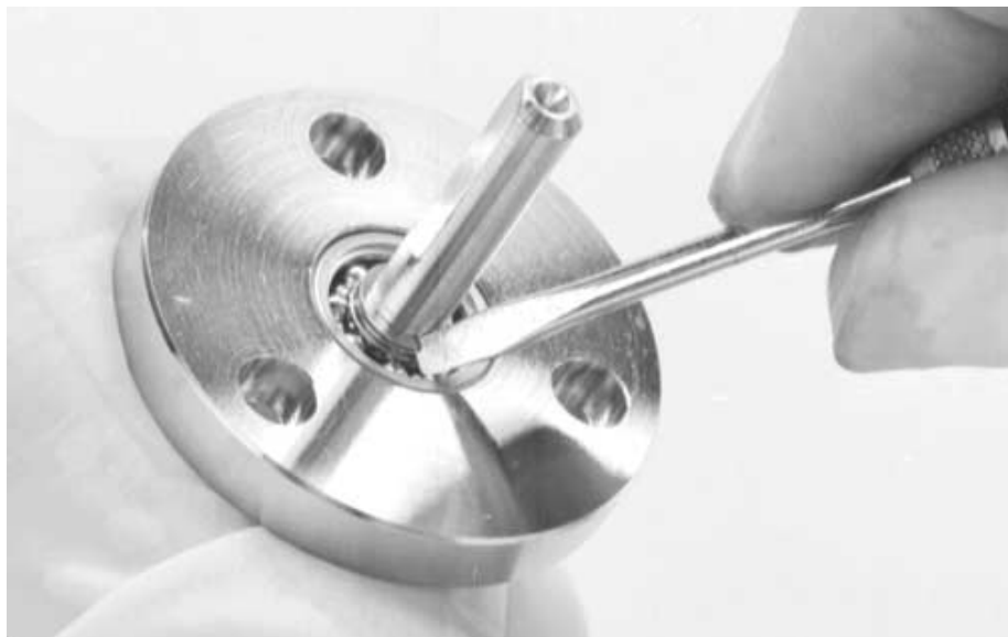
Figure 6-20. Removing the retaining ring that retains the drive shaft
