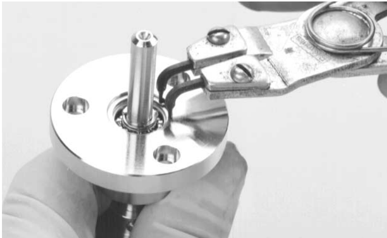
Figure 6-19. Removing the retaining ring that secures the outer crucible drive bearing in the bearing housing
