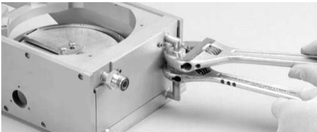
Figure 6-7. Uncoupling the water-crossover tube
