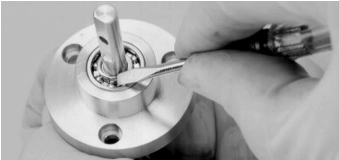
Figure 6-25. Removing the retaining ring that holds the parts of the drive shaft assembly in place
